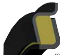
**Patented felt labyrinth seal** Includes a protective metal flinger that directs contamination away from sealing surfaces. The felt design provides a tight labyrinth seal that retains grease and acts as a filter to help exclude foreign materials. This design results in less drag and reduced heat compared to rubber contact seals. Alternate seals are available.
