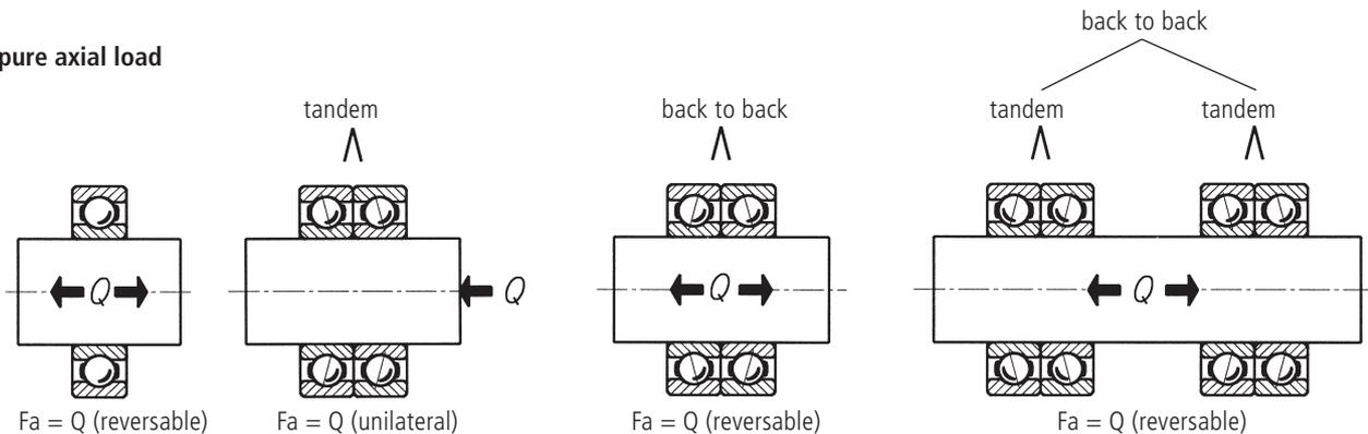
**Note:** For an axial load to be supported by several bearings, it is essential that these should be paired<sup>1</sup>, ring against ring or by means of very precise spacers.
