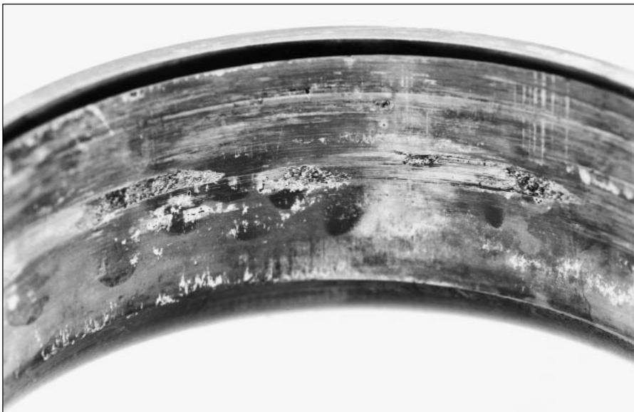
15: Seizing marks on the outside diameter as a result of outer ring creeping in the housing
