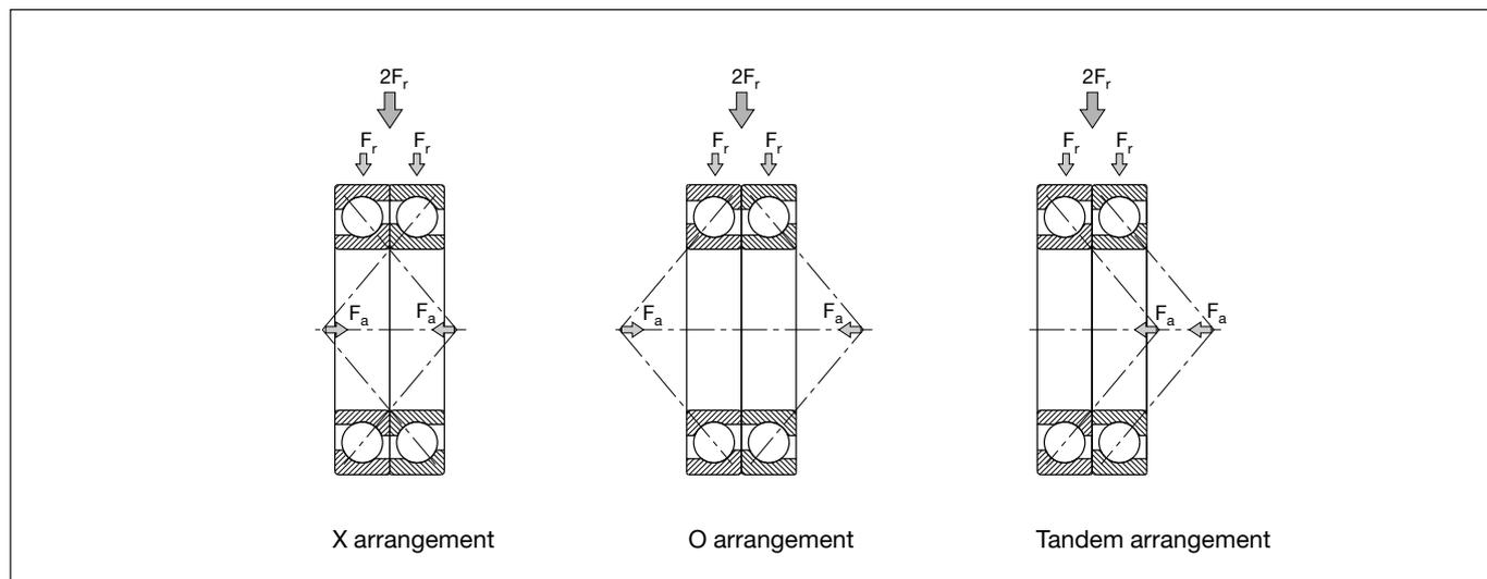
If the load carrying capacity of one single bearing is not sufficient several bearings can be mounted adjacent to one another. In this case the bearings have to be matched in such a way that as uniform a load distribution as possible and a specific clearance in the bearing set can be achieved.
