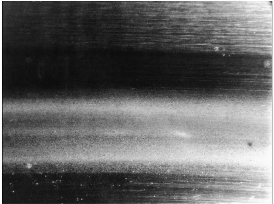
67: Wear traces can usually first be detected on the surfaces of the rolling elements
