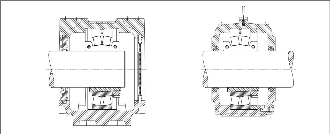
2: Easy to inspect, fast and easy mounting – the FAG split spherical roller bearing directly before mounting into an SNV housing.
