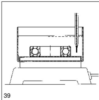
40: Heating cylindrical roller bearing inner rings in oil bath
