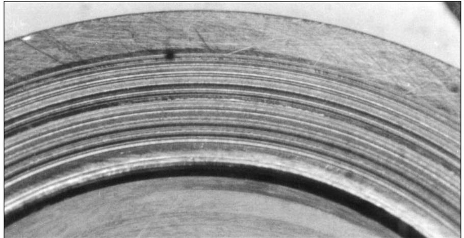
22: Seal damage due to lateral grazing
