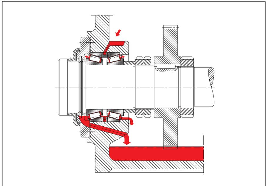
diameter. Oil is injected between the roller faces and the lip at the large race-way diameter of high-speed tapered roller
