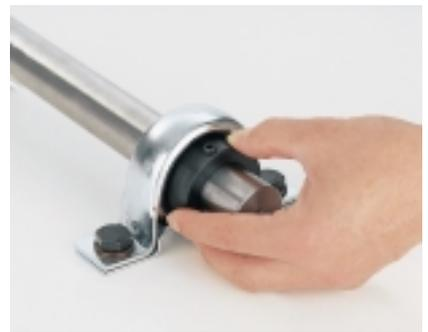
d: Localize eccentric self-locking collar by means of metal drift and hammer.
