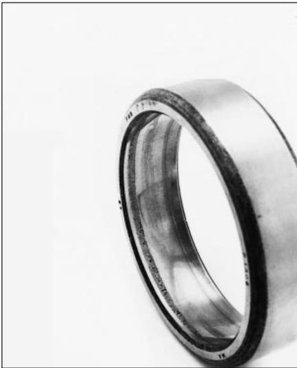
37: Development of tracks in the case of a self-aligning ball bearing with rotating inner ring under detrimental axial preload and radial load
