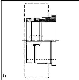
50: Larger adapter and withdrawal sleeves feature oil grooves and oil collecting grooves.
