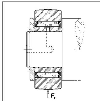
24: On mounting yoke type track rollers, the lubricating hole must be located in the unloaded zone of the raceway. The outer rings of yoke type track rollers without axial guidance must be guided by lateral backing surfaces.
