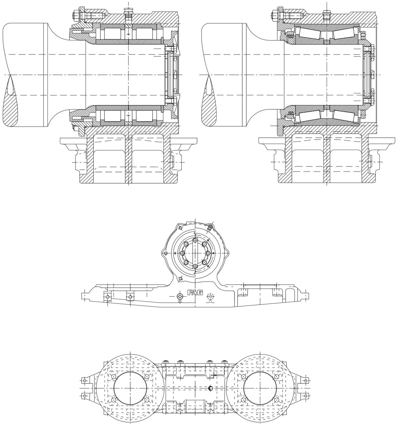
47: Axle box roller bearings of the Channel tunnel's freight engine, class 92
