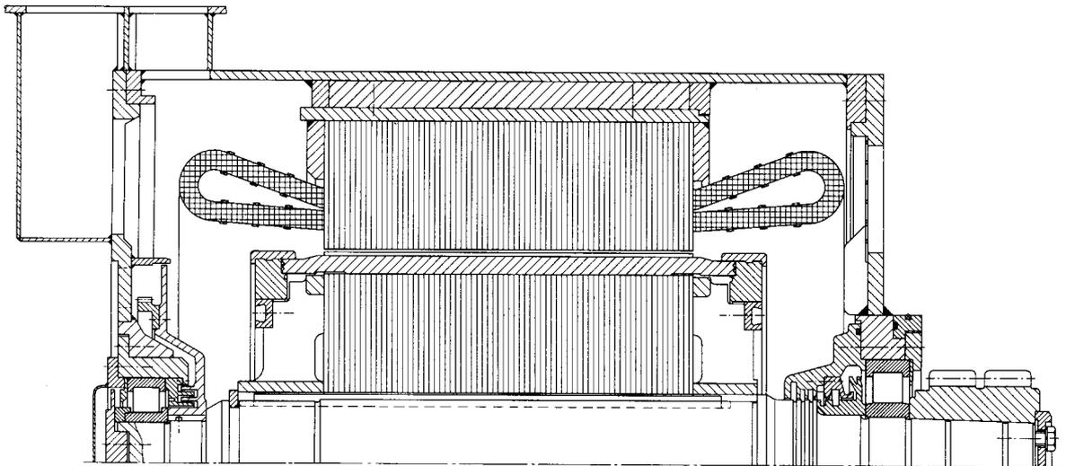
1: Traction motor for electric standard-gauge locomotive
