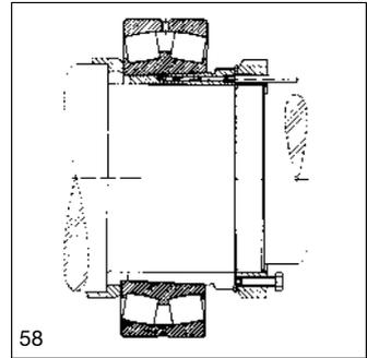
59: Bearing seated on adapter sleeve: The oil is pumped between the mating surfaces. Bolts drive the bearing up the sleeve and the radial clearance reduction is measured.
