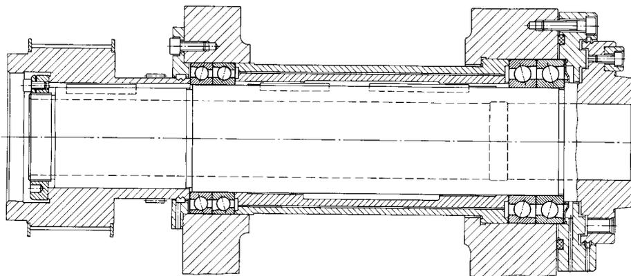
10: NC-lathe main spindle
