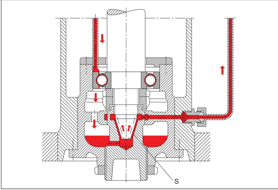
62: Oil jet lubrication with nozzles
