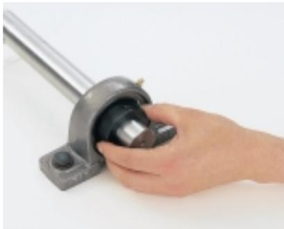
f: Localize eccentric self-locking collar by means of metal drift and hammer.
