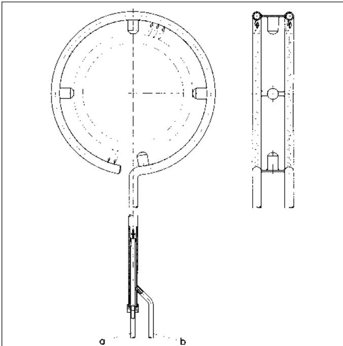
97: Ring burner for dismantling inner rings
