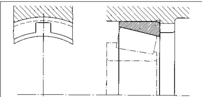
87: Slots for bearing outer ring removal
