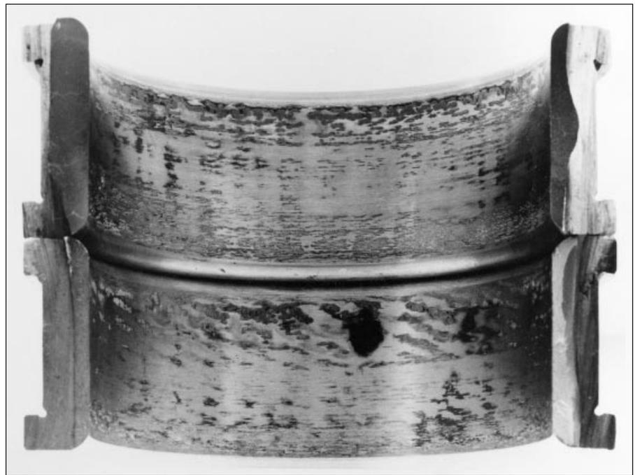
14: Fretting corrosion reveals the size of the load zone at the stationary outer ring
