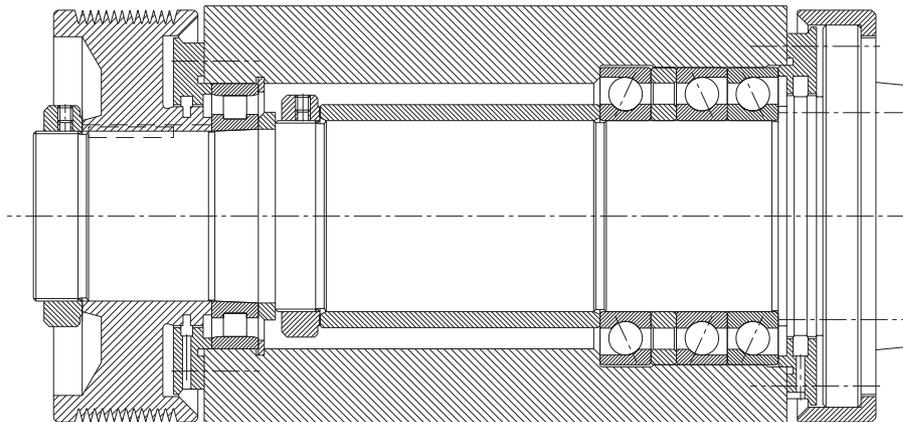
11: CNC-lathe main spindle
