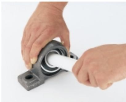
c: Push bearing unit onto the shaft together with the eccentric self-locking collar.
