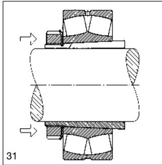
31: Press-fitting an adapter sleeve mounted spherical roller bearing with the adapter sleeve nut
