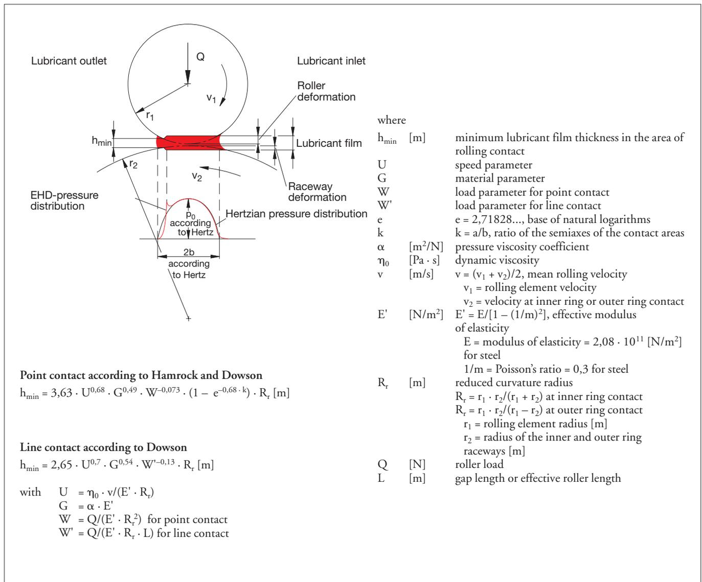
the contact surfaces are enlarged due to elastic deformation.
