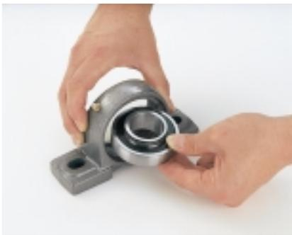
b: Swing bearing into the right position using a pin or a section of pipe; for this purpose the housing is best clamped in a vice.
