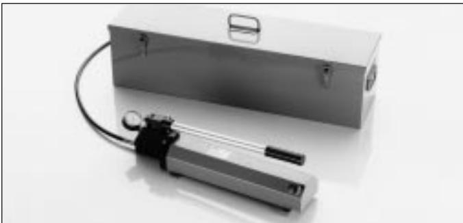
52: Hand pump set FAG 173746, consisting of a two-step piston pump (800 bar) with 3-litre oil container, manometer, extreme pressure hose and fitting (connecting thread G 1/4)
