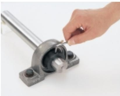
h: Series 562: tighten both threaded pins.
