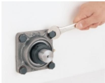
e: Manually tighten eccentric self-locking collar with a slight jerk in the direction of shaft rotation.
