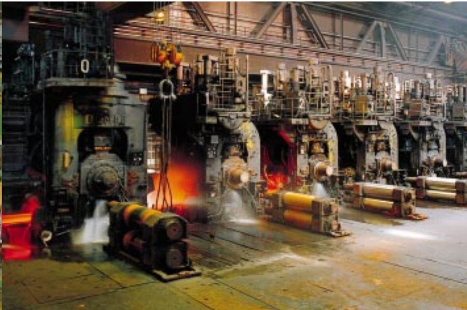
*cylindrical roller bearings – usually four-row bearings - have to do heavy labour – in the true sense of the word. This does not mean that precision goes by the board; in the case of foils the thickness tolerance is a matter of a few thousandths of a millimetre. FAG meets these demands, too. Roll forming places particularly high demands on bearing technology.*
