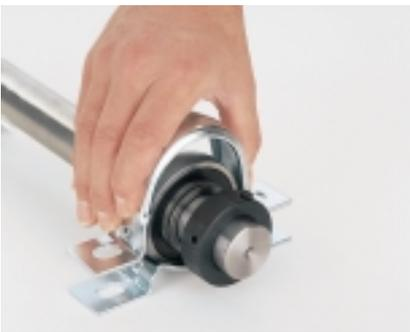
b: Slightly tighten bolts. Assemble housing and bearing at the other shaft end in the same manner. Securely tighten bolts.
