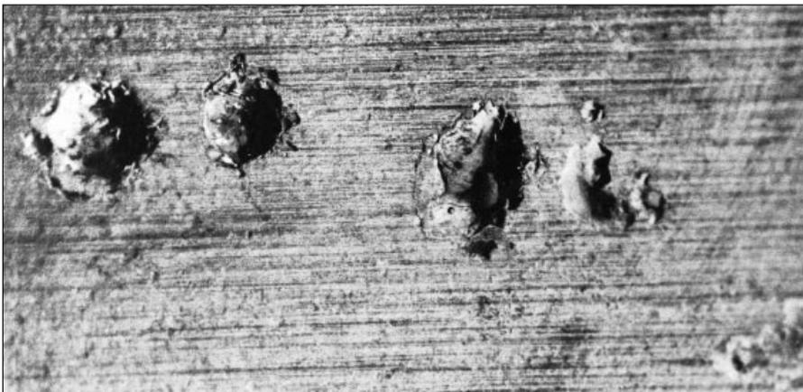
60: Fluting in the outer ring raceway of a deep groove ball bearing was caused by the constant passage of current.
