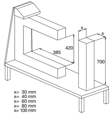
**Scope of delivery:** Device, ready for service, with ledge 100x100x700 mm and magnetic temperature sensor
