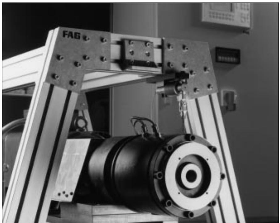
complete rolling bearings only to a limited extent. Therefore, test rigs are preferred in which rolling bearings are used as test specimens.
