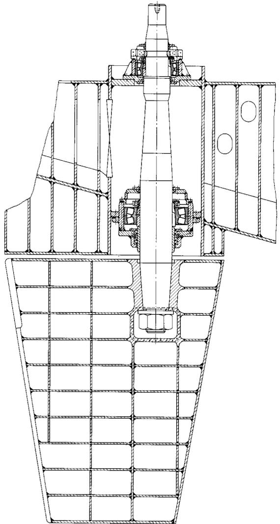
60: Spade-type rudder bearings
