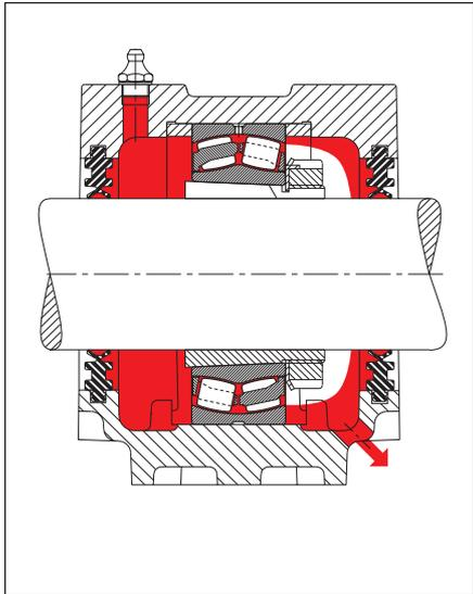
44: The pumping effect of the grease valve depends on the washer diameter.
