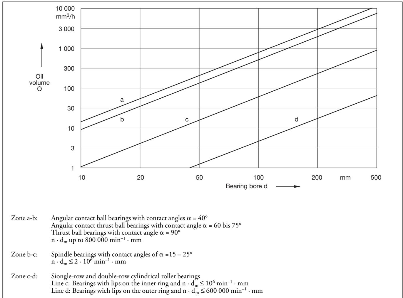
oil volume for double-row cylindrical roller bearings is shown by line d in diagram 55. Since the minimum and maximum oil volumes depend not only on the bearing but also on the oil type, the oil supply and heat dissipation it is not possible to furnish a general rule for determination of the speed index and the optimum small oil quantities. The viscosity of the oil selected should result in a viscosity ratio of  $\kappa = 2$  to 3.
