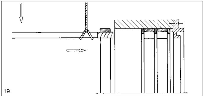
Heavy bearing outer rings with sliding fit can be mounted with a mounting lever (Fig. 19).
