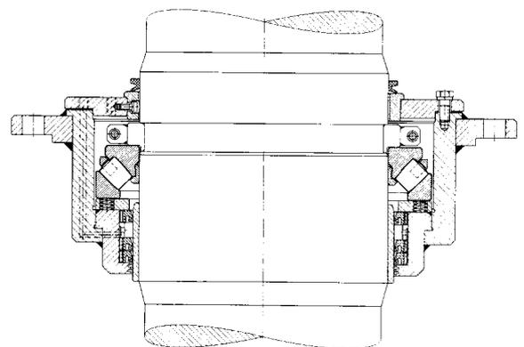
59: Rudder carrier bearing FAG RS9284W.1.....
