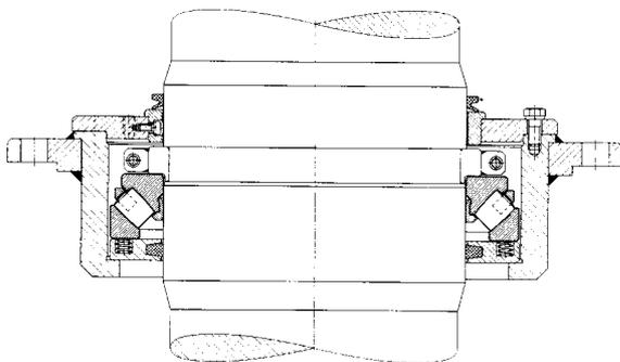
58: Rudder carrier bearing FAG RS9284N.1.....
