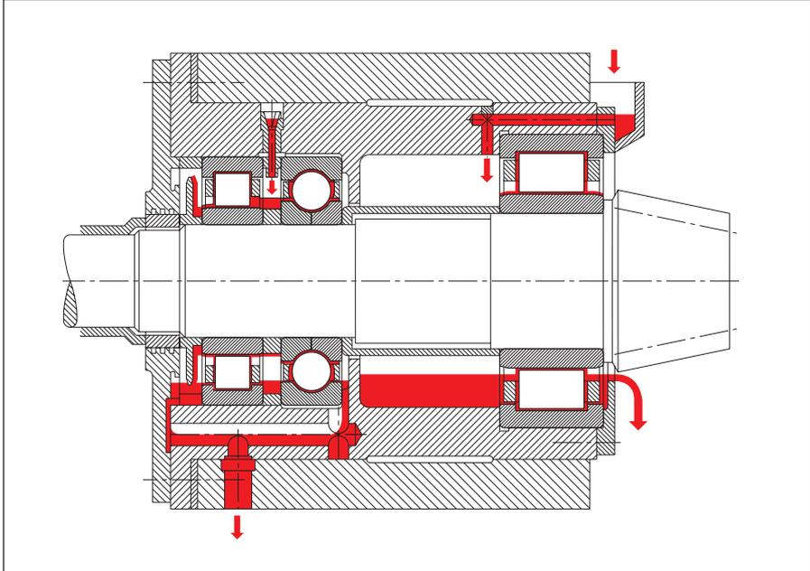
63: Oil jet lubrication: Oil supply at either side of a high-speed tapered roller bearing
