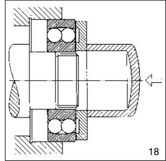
In some self-aligning ball bearings, the balls protrude beyond the rings. In such cases, the disk must be relieved (Fig. 18).
