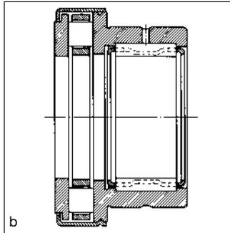
23: Combined needle roller - thrust ball bearings and needle roller - cylindrical roller thrust bearings with dust shield must be pressed into the housing.
