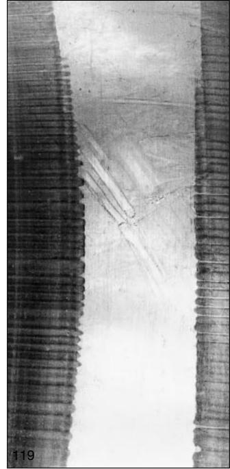
In the case of overlubrication, the lubricant heats up due to the churning action and loses its lubricity. Overheating, i. a. catastrophic failure of the bearing, may be the result. Prevent lubricant retention within the bearing, especially for high-speed bearings.
