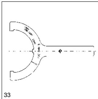
33: Double hook spanner with engraved rotation angles for fitting self-aligning ball bearings
