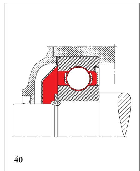
little grease remains in the bearing at the side facing the grease valve. This can be avoided by displacing the gap between the rotating grease valve and its stationary counter part nearer to the shaft. A normal grease valve where the gap is at bearing outer ring level (fig. 44a) has a strong
