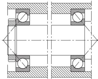
Adjusted bearing arrangement (X arrangement)
