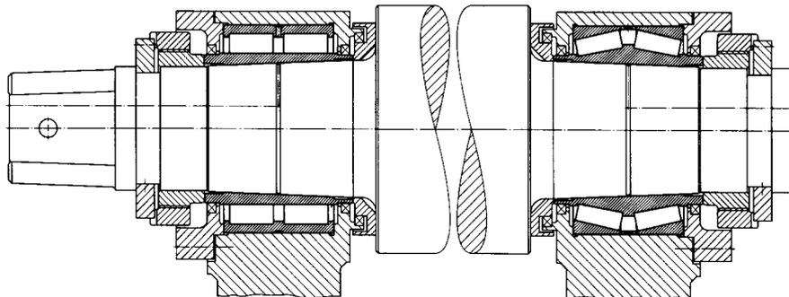
108b: Bearing mounting of horizontal rolls for stands in which section steel is finish-rolled
