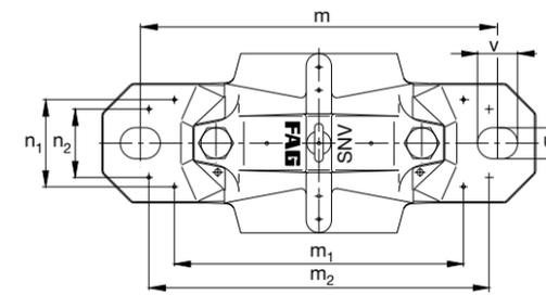
Bearing with tapered bore and adapter sleeve
