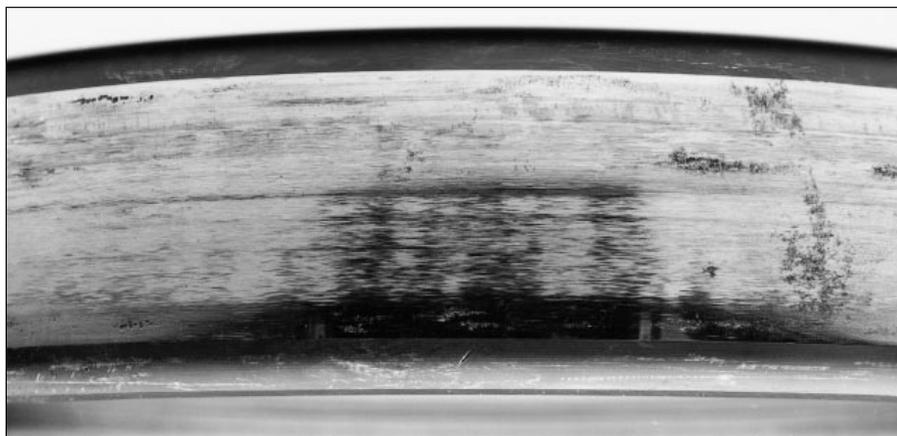
17: Circumferential scoring and cold welding at the inner ring faces as a result of inner ring creeping on the shaft
