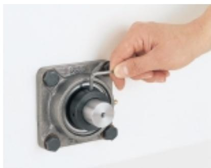
h: Series 562: tighten both threaded pins.
