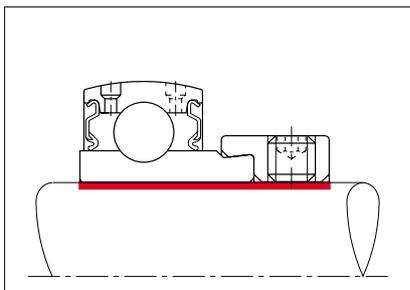
The bearings are fastened on the shaft either by means of eccentric self-locking collars or two threaded pins.
