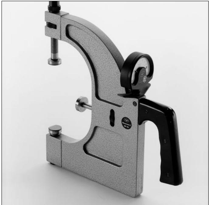
Another useful instrument is the snap gauge shown in fig. 3. It functions as a comparator and its correct setting is checked with master rings. These master rings are supplied by FAG for each diameter.
