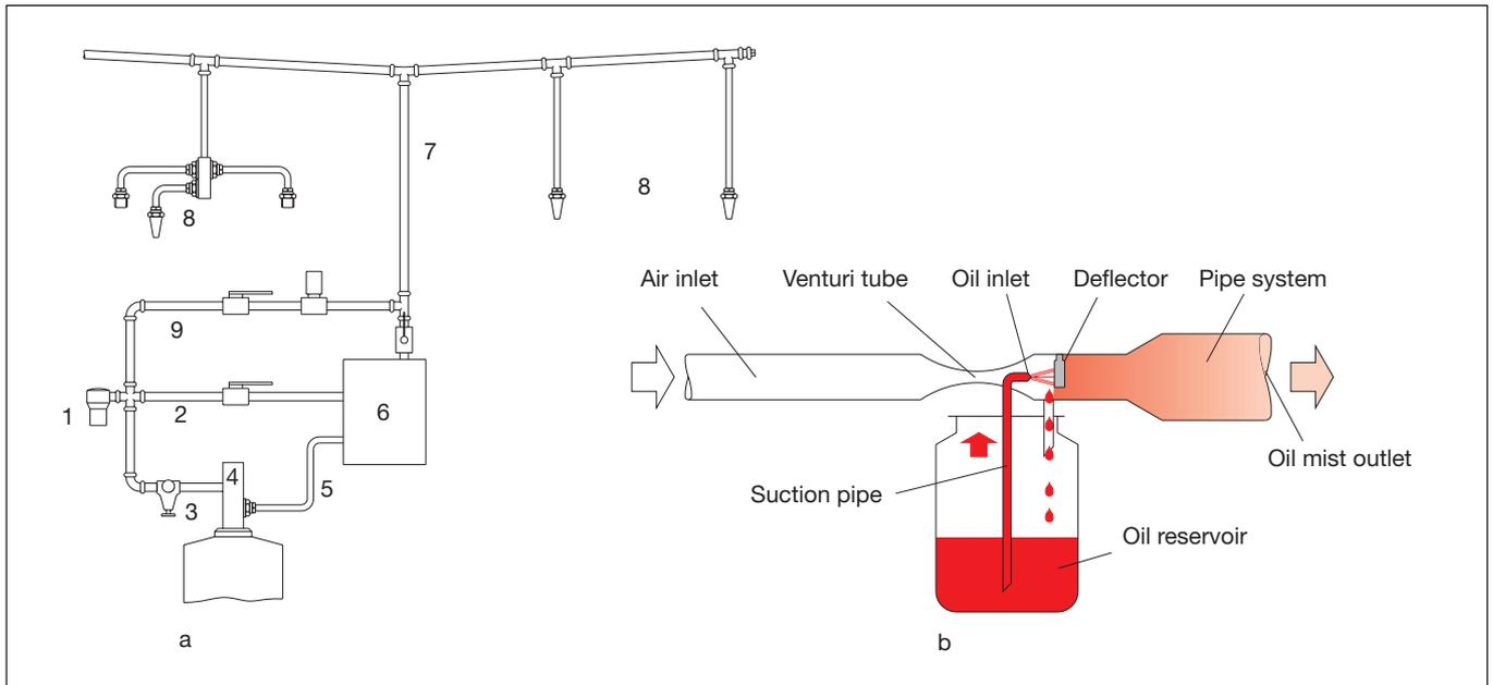
24a: Schematic drawing of an air-oil lubrication system (according to Woerner). 1 = automatic oil pump, 2 = oil pipe, 3 = air pipe, 4 = oil-air mixing unit, 5 = oil metering element, 6 = air metering element, 7 = mixing chamber, 8 = oil-air pipe.
