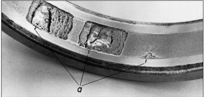
111: Fractured lip of a barrel roller bearing inner ring driven up its seat by hammer blows
