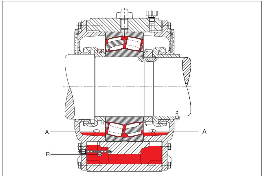
59: Oil circulation in bearings with conveying or pumping effect
