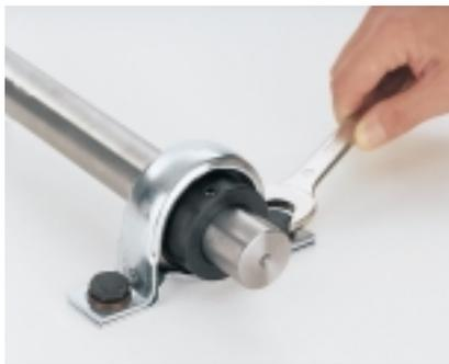
c: Manually tighten eccentric self-locking collar in the direction of shaft rotation.
