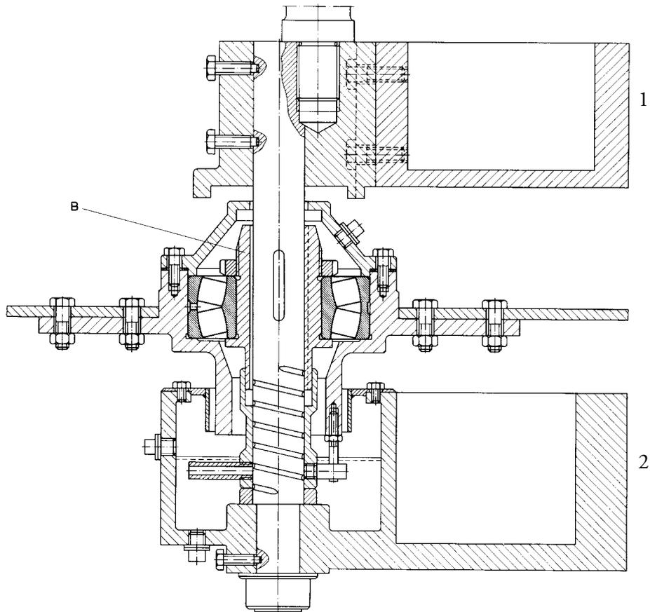
Printing quality is created in the heart of a printing press, the printing group with its main cylinders. Plate cylinders, blanket cylinders and impression cylinders are, therefore, guided in rolling bearings which are particularly low in friction and which have a high degree of running accuracy and radial rigidity.
