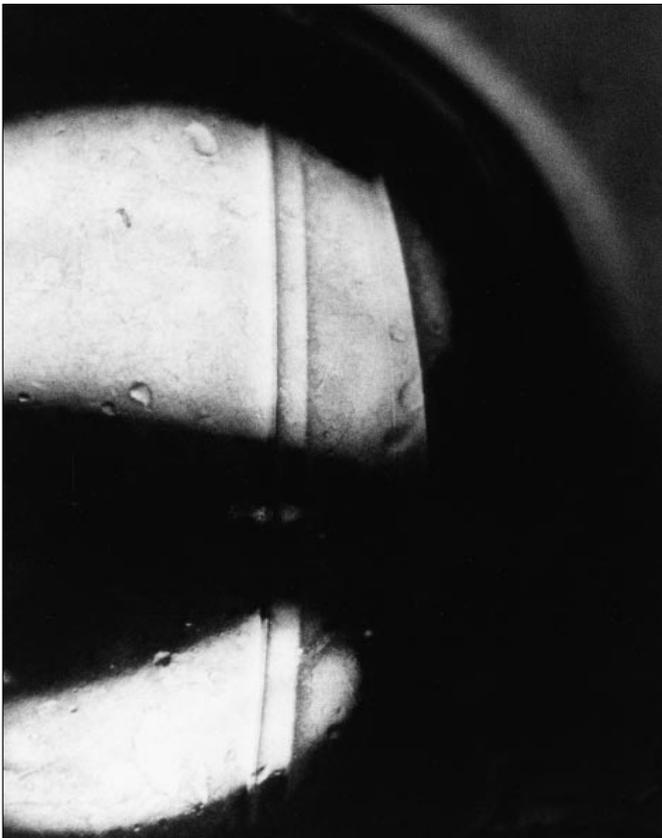
62: Ball with "woolen balls" of notches caused by long-term changing load
