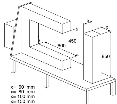
**Scope of delivery:** Device, ready for service, with ledge 150x150x850 mm, and magnetic temperature sensor.
