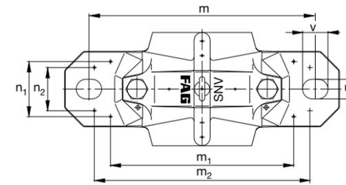
Bearing with tapered bore and adapter sleeve
