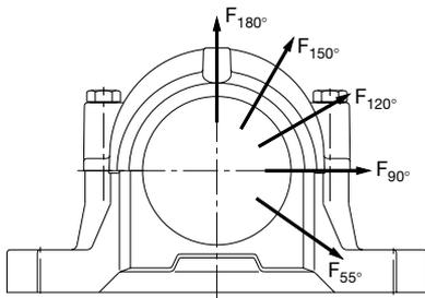
For compensation of the housing breaking load value a safety factor of 6 is recommended.
