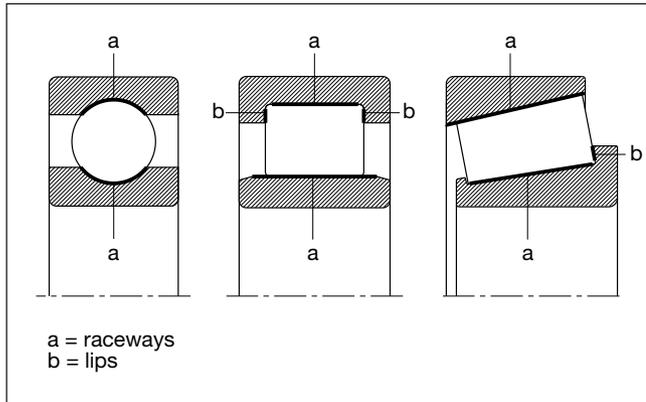
The two rings of **separable** rolling bearings can be mounted separately. This is of advantage if both bearing rings have to be mounted with a tight *fit* (see page 28).
