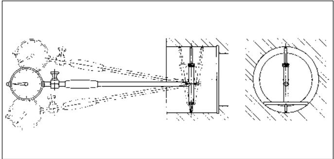
**Check diameter and cylindricity of shaft and housing seats**
