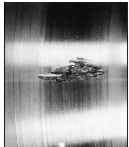
51: Wear in diverse areas can change the geometry of the components in rolling contact to such an extent that local overload leads to fatigue
