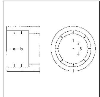
Unless otherwise specified in the shop drawing, the cylindricity tolerance should not exceed half the diameter tolerance (two-point measurement).
