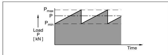
The mean value of the equivalent dynamic load may **not** be used for the *adjusted rating life calculation* (page 12ff). Rather, the *attainable life* under constant conditions has to be determined for every operating time.
