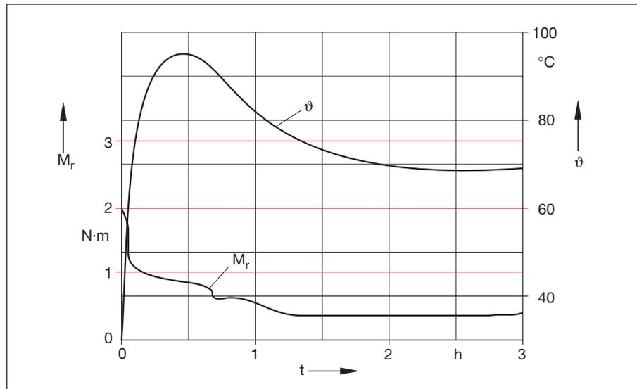
These effects are even more intensive, the larger the grease quantity in and beside the bearing and the more the movement of the grease out of the bearing is obstructed. They can be counteracted by an interval lubricant supply system with accordingly specified downtimes for cooling such as is used for spindle bearings in machine tools.
