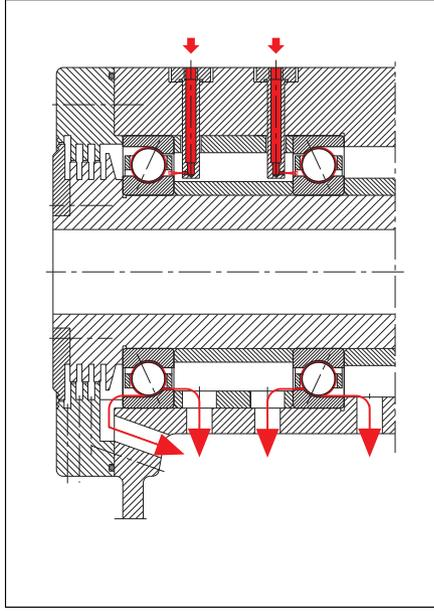
61: Oil thrown off is collected in a pocket and fed through grooves into the cylindrical roller bearing.
