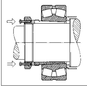
For larger bearings, considerable forces are required to tighten the nut. In such cases, the mounting nut with thrust bolts shown in Fig. 34 facilitates mounting.
