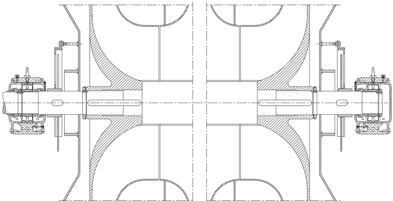
118: Rotor mounting of an exhauster
