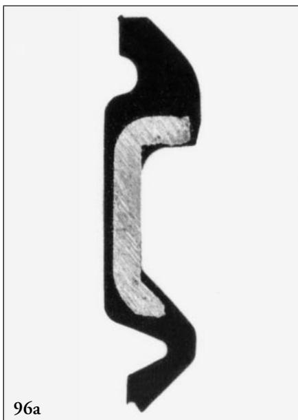
96: Cross section of a seal.
