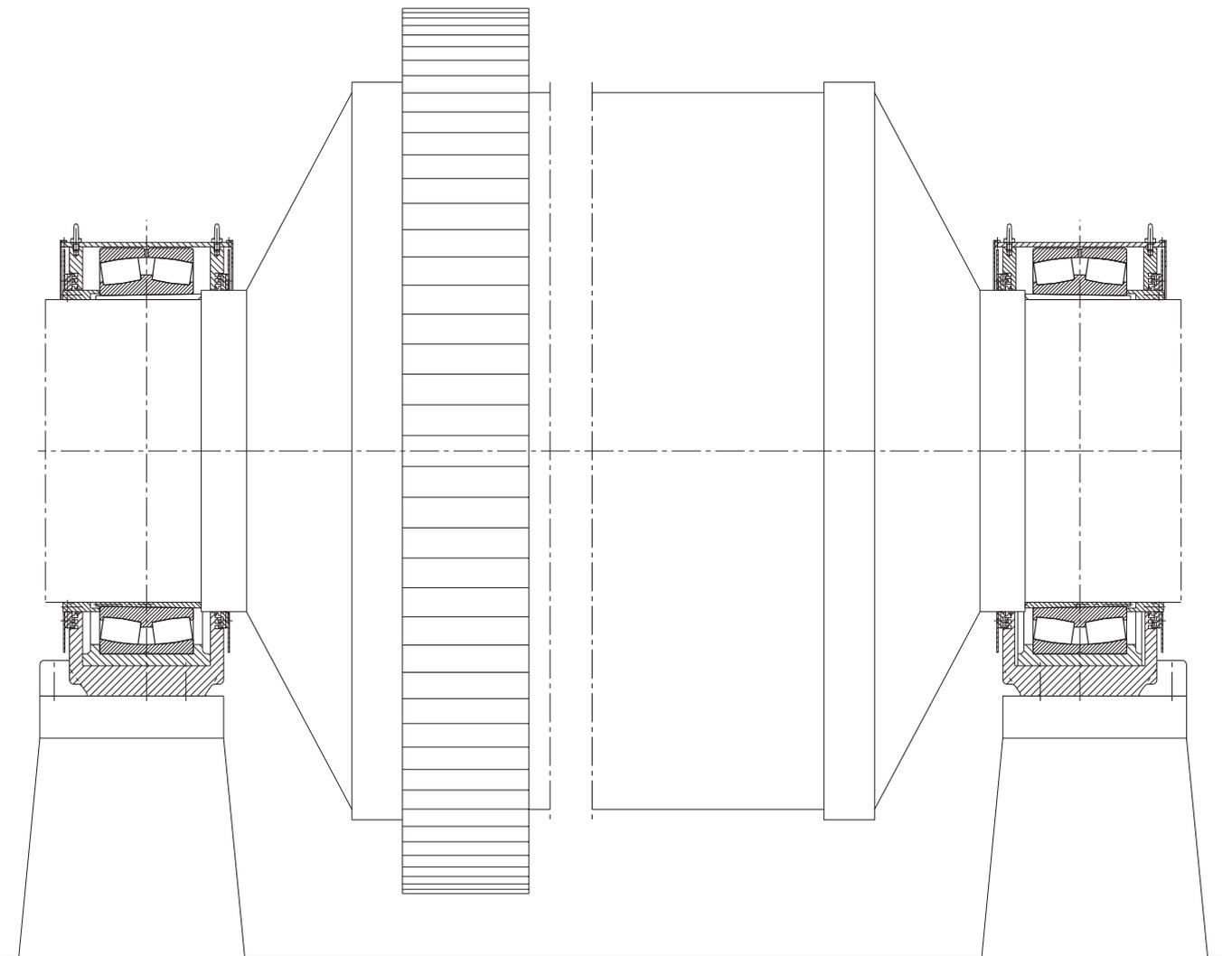
95: Ball tube mill mounting
