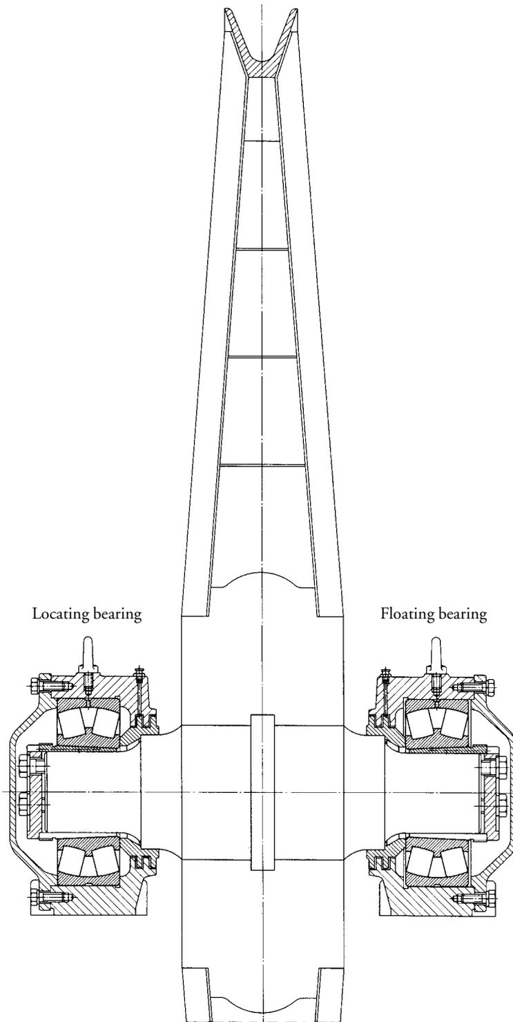
75: Rope sheave (underground mining)
