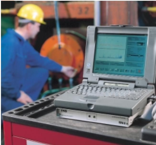
FAG offers a proactive maintenance program to assure early detection of problems. We can then schedule corrective actions before a catastrophic failure occurs.
