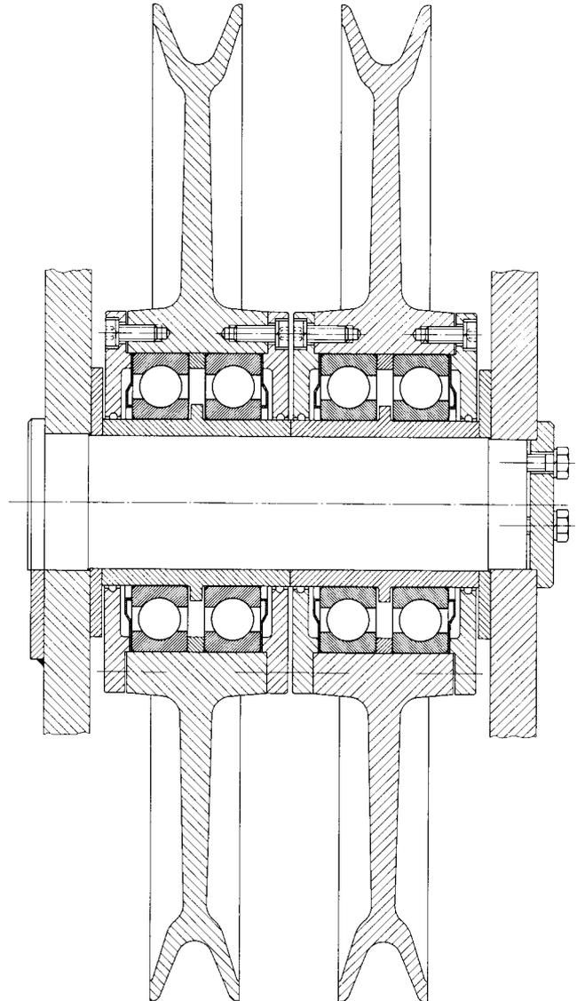
76: Rope pulleys with deep groove ball bearings
