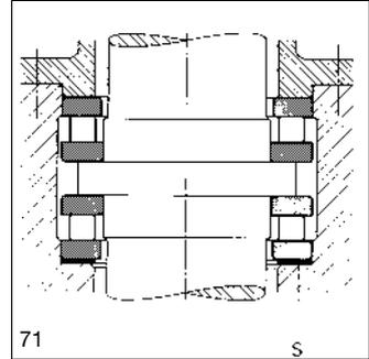
This is a field-proven method of adjusting wheel bearings requiring no special tools. There are other methods which, however, necessitate mounting tools and measuring instruments. They are primarily intended for batch mounting.
