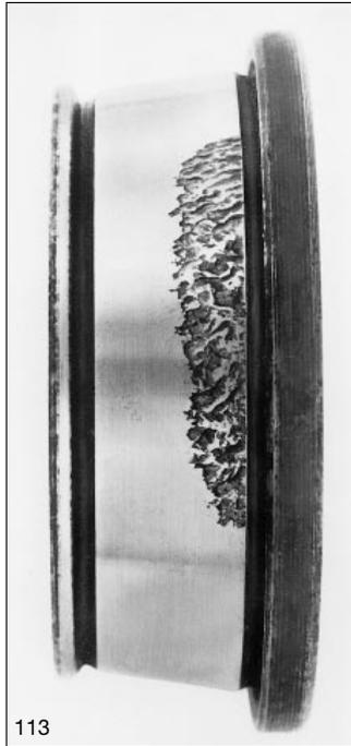
113: One-sided flaking caused by off-square mounting of a stationary tapered roller bearing cone
