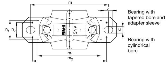
Bearing with tapered bore and adapter sleeve
