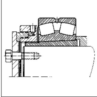
Adapter sleeves can be released with a hydraulic nut provided the bearing rests against an angular support ring. The nut should take support on a plate or the like (Fig. 92).
