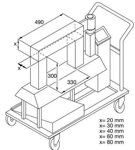
**Scope of delivery:** Device, ready for service, with slewing ledge 80x80x490 mm, and magnetic temperature sensor
