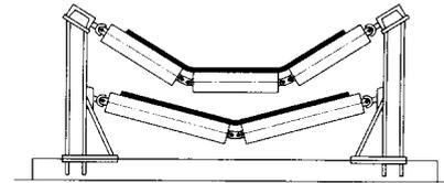
Fig. 86 shows idler garlands connected by chain links. These idlers are part of a conveying installation for rock phosphate. The bearings fitted are deep groove ball bearings FAG 6303.2ZR.C3.
