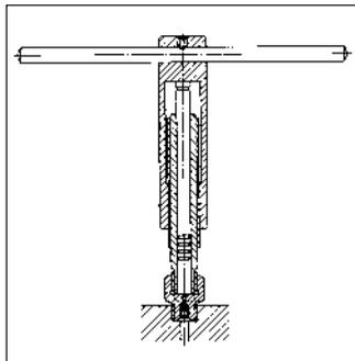
51: Oil injector and valve nipple for connecting thread G 3/8:
