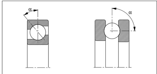
*Ball bearings* and *roller bearings* with symmetrical rolling elements have identical contact angles at their inner rings and outer rings. In roller bearings with asymmetrical rollers the contact angles at the inner rings and outer rings are not identical. The equilibrium of forces in these bearings is maintained by a force component which is directed towards the lip.
