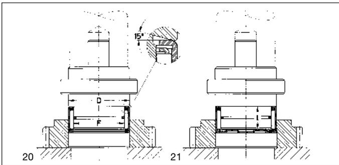
Drawn cup needle roller bearings are pressed into the housing with a mounting mandrel.
