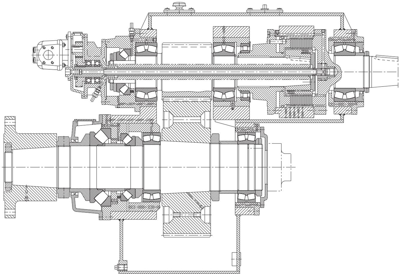
28: Bearing arrangement of a marine gear
