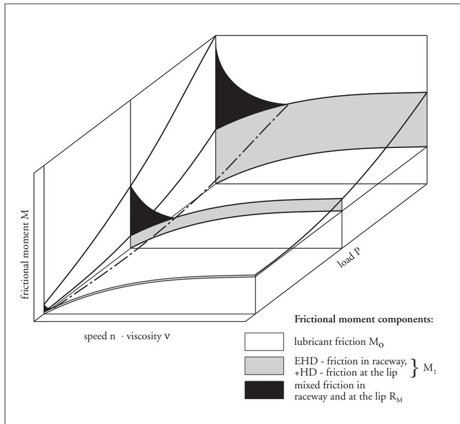
$\nu$  [mm<sup>2</sup>/s] operating viscosity of the oil or grease base oil (fig. 5, page 6)
