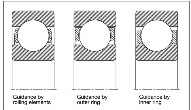
Under normal operating conditions, the cage design specified as the standard design is usually suitable. Within a single bearing series the standard cages may differ depending on the bearing size, cp. section on "Spherical roller bearings". Where specific operating conditions have to be accommodated, a cage custom-tailored to these conditions has to be selected.
