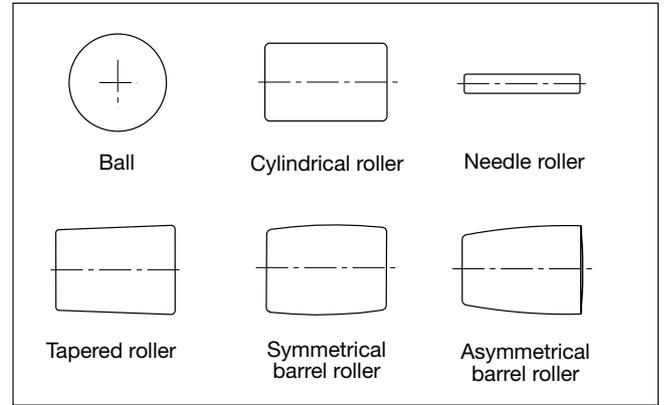
The rolling elements' function is to transmit the force acting on the bearing from one ring to the other. For a high load carrying capacity it is important that as many rolling elements as possible, which are as large as possible, are accommodated between the bearing rings. Their number and size depend on the cross section of the bearing.
