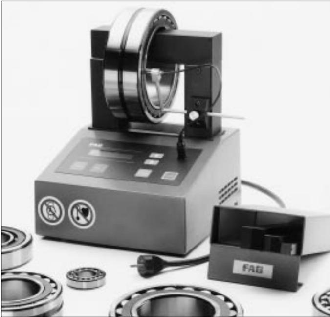
43,44: The induction heating devices ensure fast, clean and secure heating up to mounting temperature.
