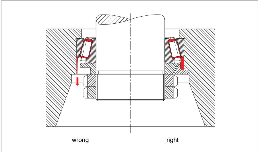
42: The grease is fed through the bearing outer ring.
