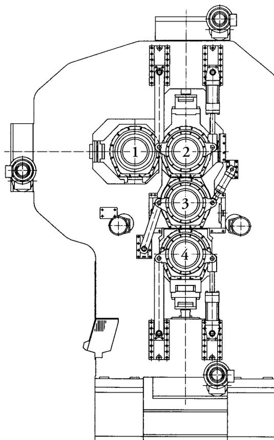
cal roller bearings (dimensions 500 x 650 x 130 mm) and deep groove ball bearings FAG 61996M.P65. At the *locating bearing* end the radially relieved deep groove ball bearing accommodates only axial guiding loads.
