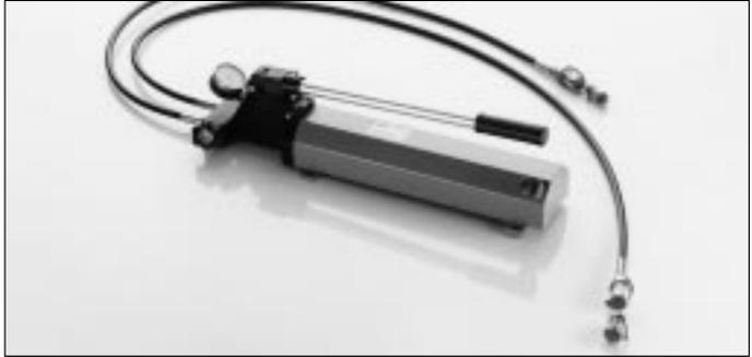
54: Hand pump set FAG 173748, consisting of a two-step piston pump (1500 bar), with 3-litre oil container, manometer, extreme pressure hose and fitting (connecting thread G 1/4)
