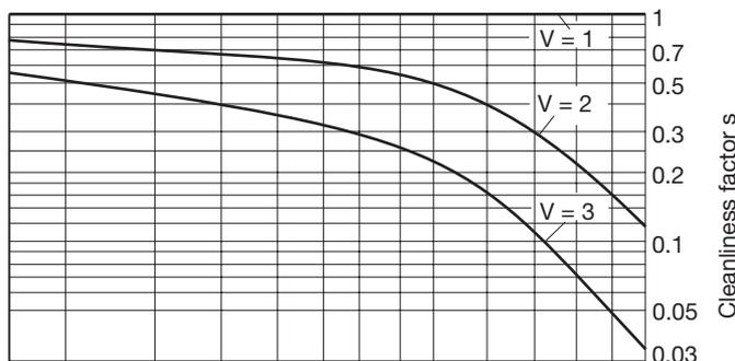
A cleanliness factor  $s > 1$  is attainable for full-complement bearings only if wear in roller/roller contact is eliminated by a high-viscosity lubricant and utmost cleanliness (oil cleanliness according to ISO 4406 at least 11/7).
