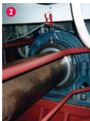
2. A typical installation of a Cooper BCP on a propulsion shafting application.
